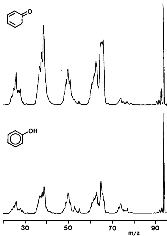
Figure 1. ^+NR^+ (Hg(90%T)/O 2 (50%)) mass spectra of A)cyclohexa-2,4-dienone and B)phenol radical cations.
