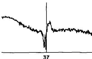
Figure 4. Effect obtained when normal peak subtraction at mass 37 of n-hexane is slightly off-set on the mass scale.
